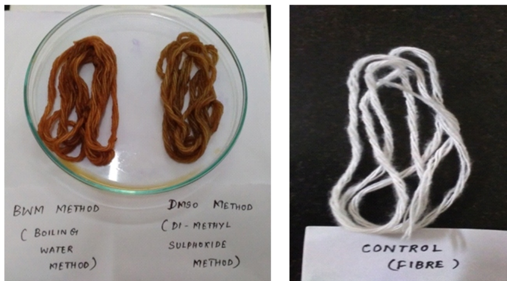
Fig 1: Comparison of the control fibre (undyed) with that of the dyed fibre
