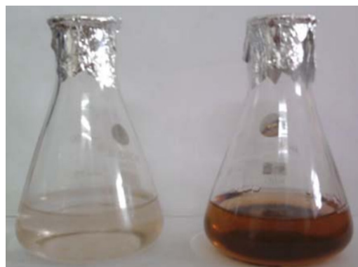
Figure 1: Synthesis of silver nanoparticles. Synthesis confirmed by colourless to yellowish brown colour solution.
