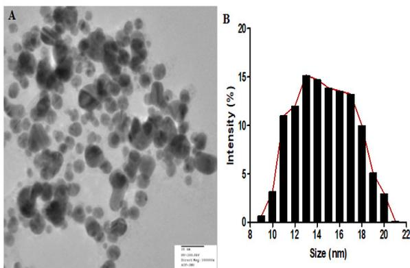
Figure 2: (A) TEM micrograph recorded from a drop-coated film of gold aqueous solution formed by the reaction of 1 mM  $\text{HAuCl}_4$  and 5% *Dictyota dichotoma* leaf broth. The scale bar corresponds to 20 nm. (B) Gold nanoparticles size distribution histogram.
