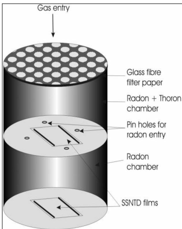
Figure 2: Schematic diagram of Single-entry Pin-hole dosimeter.<sup>[8]</sup>
